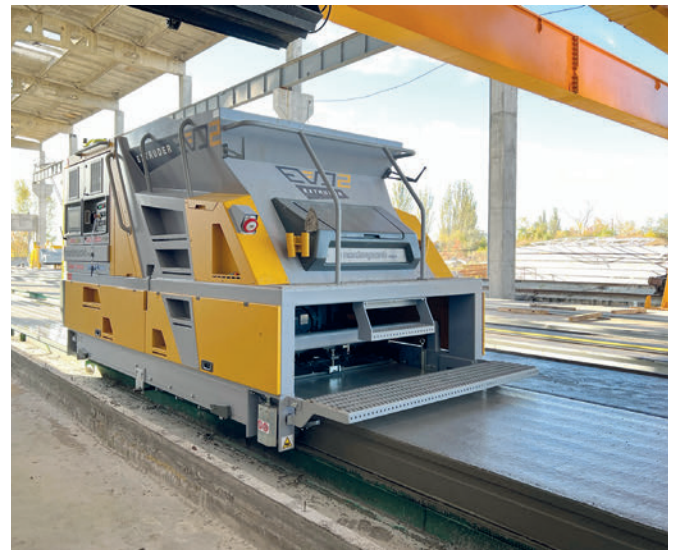
Casting of hollow core slabs 220mm high with EVO2 Extruder
