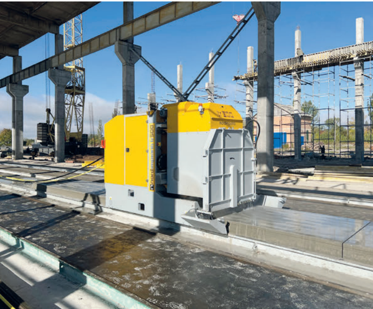
Automatic cross-cut saw
