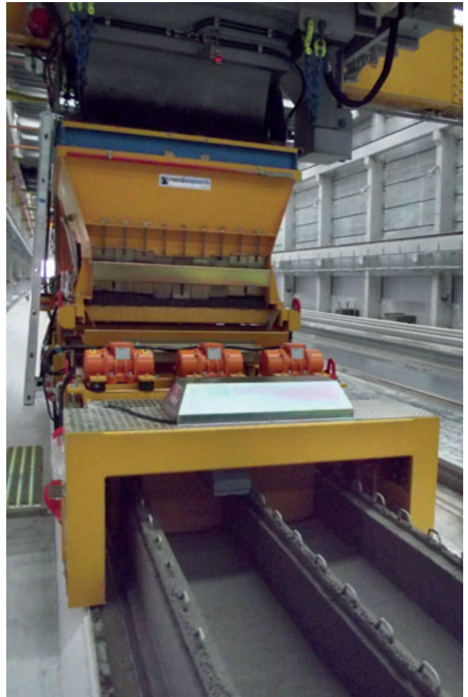
Triple Ribbed Slabs during casting phase with Nordimpianti's Slipformer machine showing the protruding steel coming out 100 mm from the element
