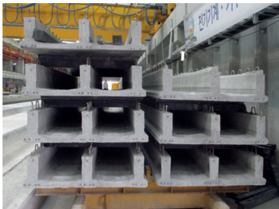
The new pre-stressed Triple Ribbed Slab concrete floor element
