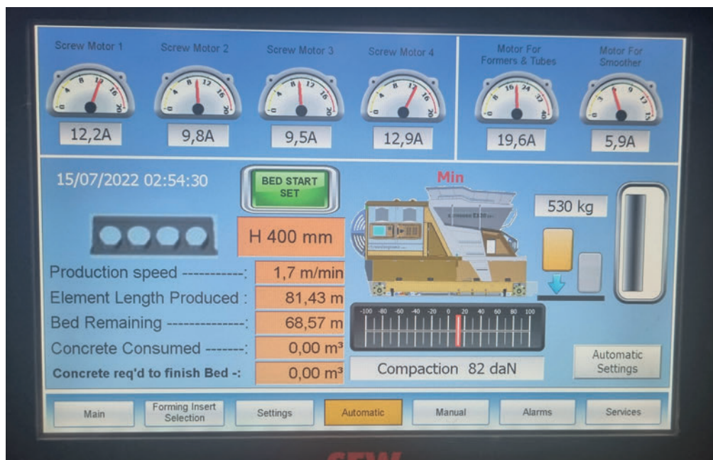
HMI operating panel of the extruder machine showing a production speed of 1.7m/min for 400mm hollow core slabs
