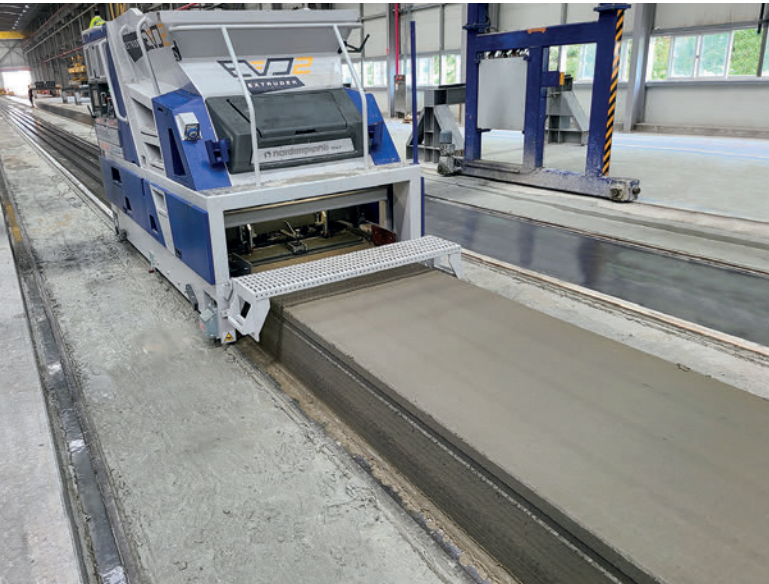
Extruder EVO2 during the first bed casting of 400mm high hollow core slabs
