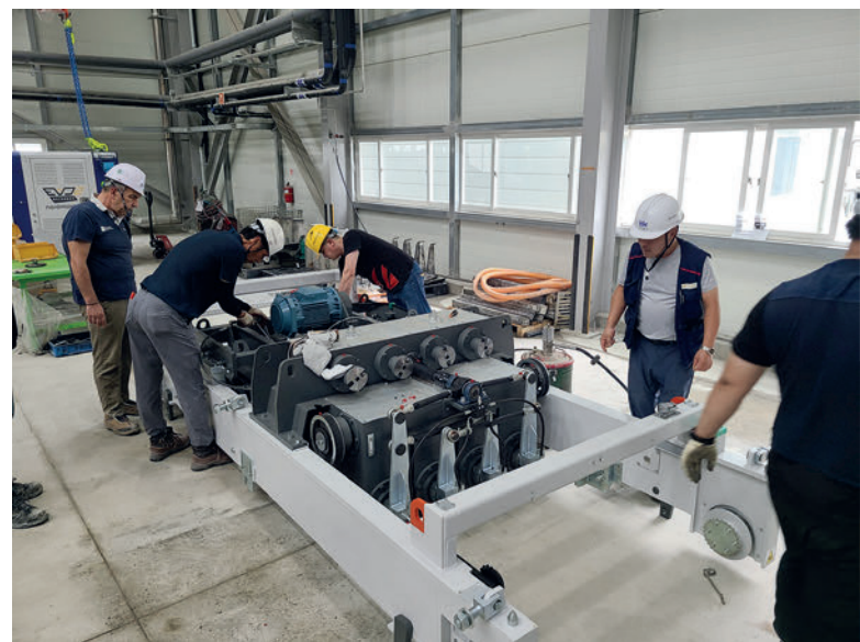
GPC's personnel appreciating the permanent oil bath gearbox transmission on arrival at the plant
